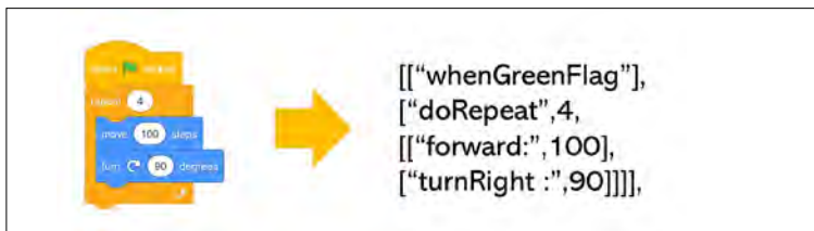
Fig. 3. Example of how information from a Scratch script is represented in a JSON file.
