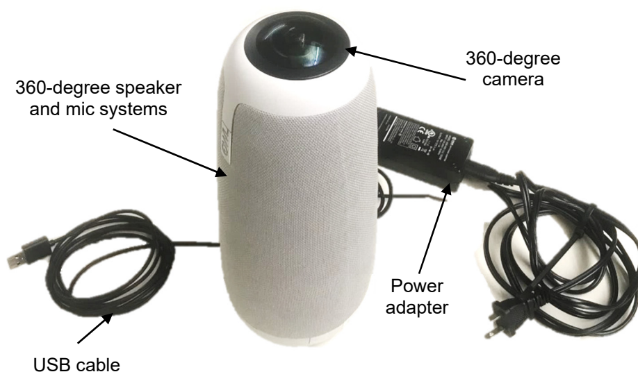
Figure 2. Meeting Owl Pro device and its different components.
