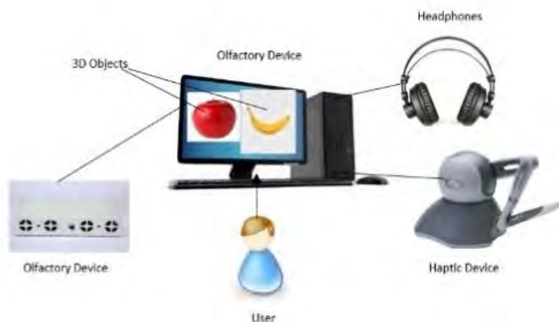
Figure 17: Proposed framework for virtual edutainment environment using haptic, audio, and olfactory Sensors
