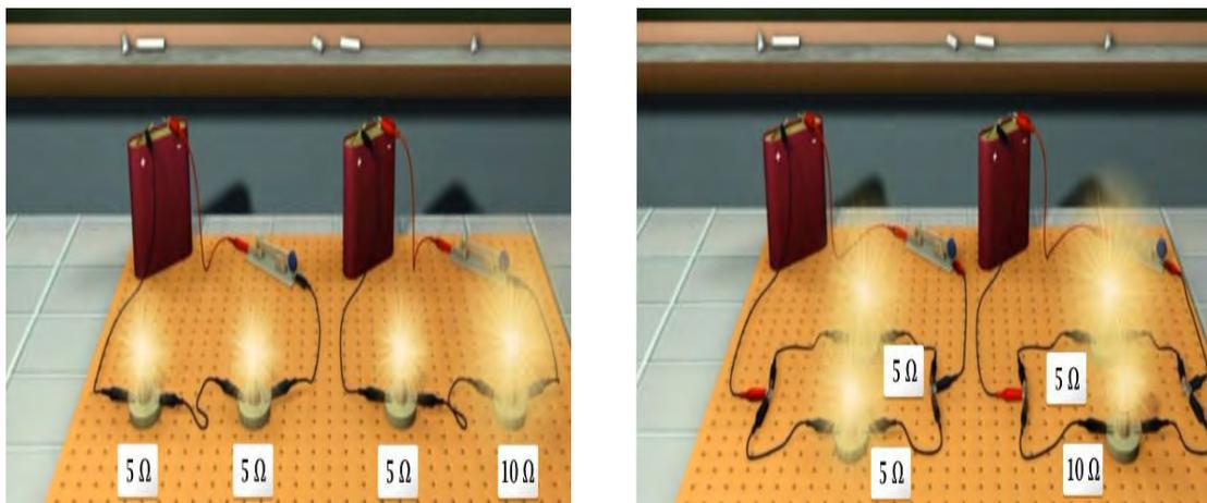
Figure 2. Brightness connecting in series and parallel bulbs
