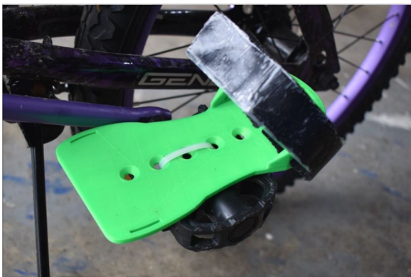
Figure 3 Adapted bicycle pedal (Thing 1560036)
