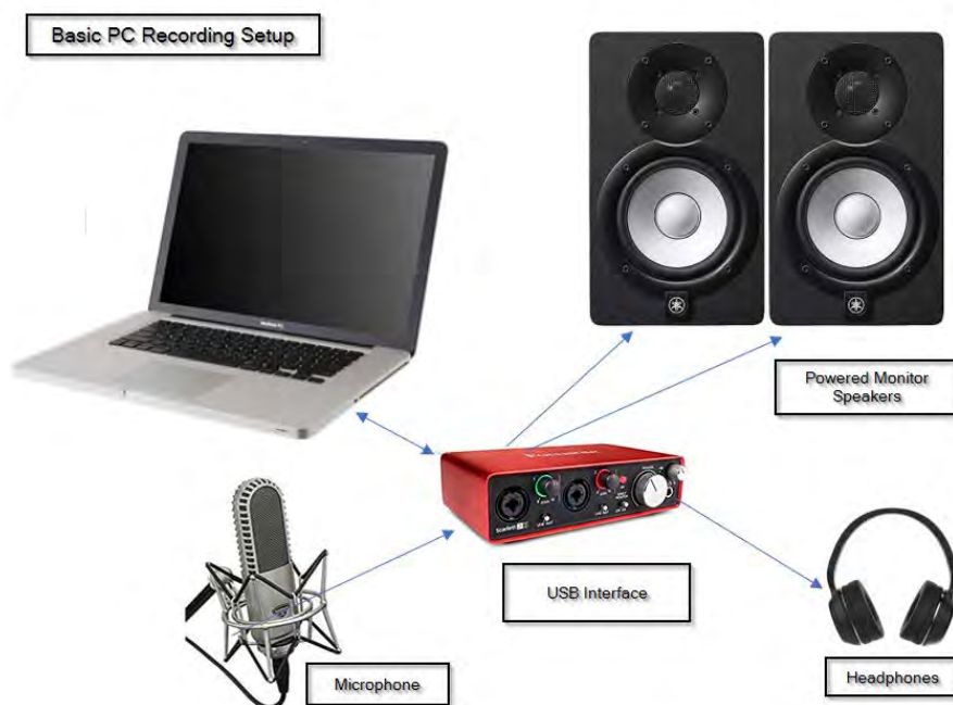
Figure 2. Illustration of basic computer recording setup using a USB interface.
