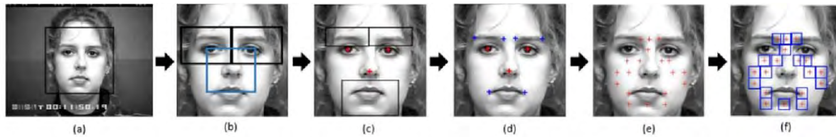
Figure 1. Framework for automated facial landmark detection and active patch extraction (Happy & Routray, 2014).
