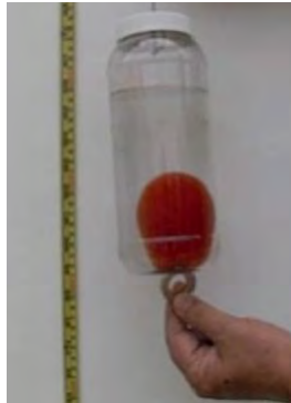
Fig. 5. The neodymium magnet holding the tomato at the bottom before the bottle was free to fall
