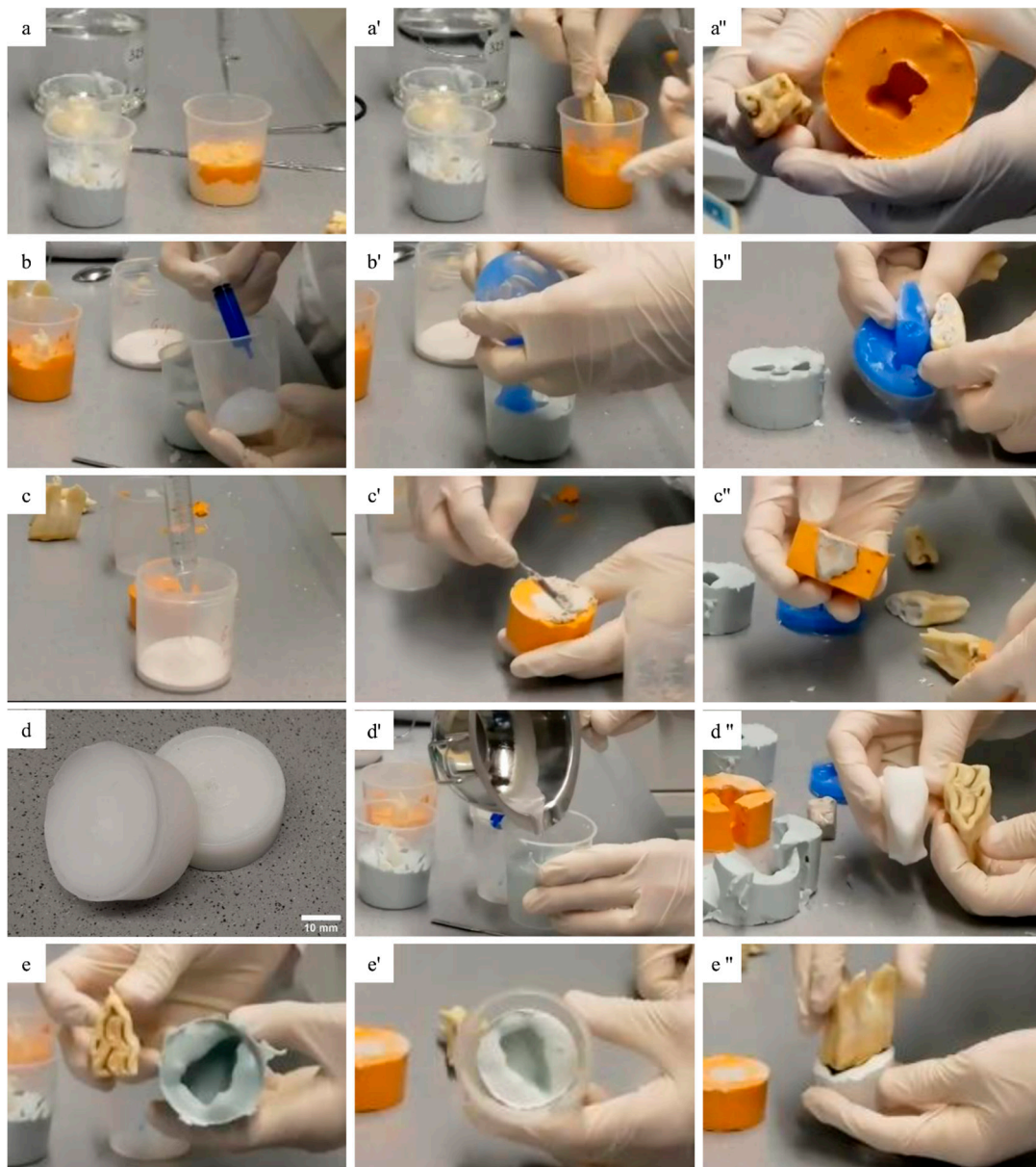
Figure 4. Screenshots taken from the video stream during preparation of tooth impressions and the fabrication of tooth models from various modeling materials. Alginate impression material (orange and cyan) during mixing with water (a), impression of an equine molar (a'), and after the demolding of the tooth (a''). Mixing the two-component polyaddition silicone (b), pouring it into the alginate negative (b'), and demolding the silicone model (b''). The plaster is mixed with water (c), the alginate negative is filled with the plaster (c'), and the plaster model is demolded with the loss of the alginate mold (c''). Wax before heating to approx. 70 °C (d) to fill the alginate negative (d') and comparison of the wax model with the original tooth after demolding with loss of the alginate mold (d''). Comparative presentation of the tooth and alginate mold immediately after demolding (e), after storage at room temperature for >4 weeks (e'), and the comparison of the dried alginate mold with the originally demolded tooth (e'').
