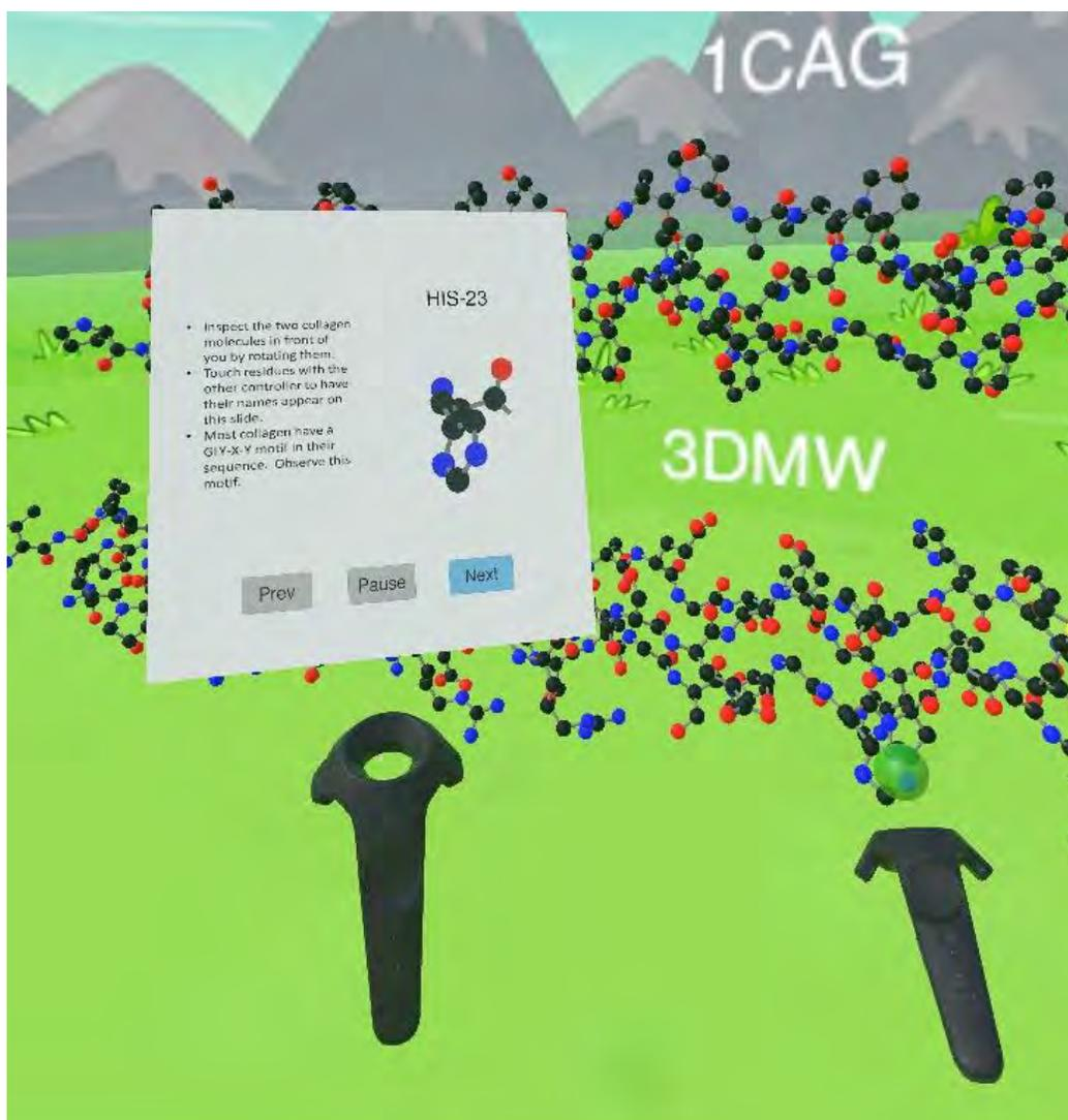
Figure 4 - VR Controls: The two standard Vive controllers served different functions. The left controller displays the current slide and is used to navigate the interactive slide elements. The right controller is used to manipulate the proteins, change visualizations, and make measurements. Here a student is using the right controller to select a residue which is then displayed on the left controller.
