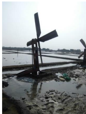
Figure 4 “Kitiran” as a traditional tool that is used to move water into salt fields
