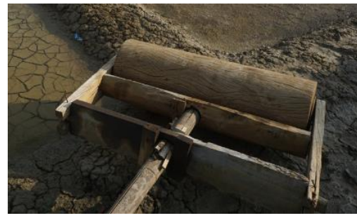
Figure 2 “Glondongan” as a traditional tool that is used to compact and flatten a salt pond plot
