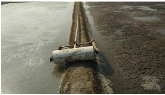
Figure 2 “Glondongan” as a traditional tool that is used to compact and flatten a salt pond plot
