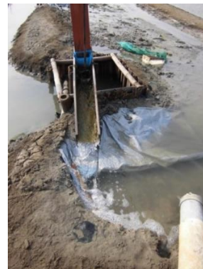
Figure 4 “Kitiran” as a traditional tool that is used to move water into salt fields
