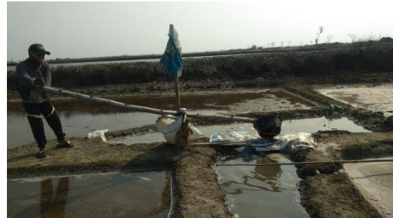
Figure 2 “Glondongan” as a traditional tool that is used to compact and flatten a salt pond plot
