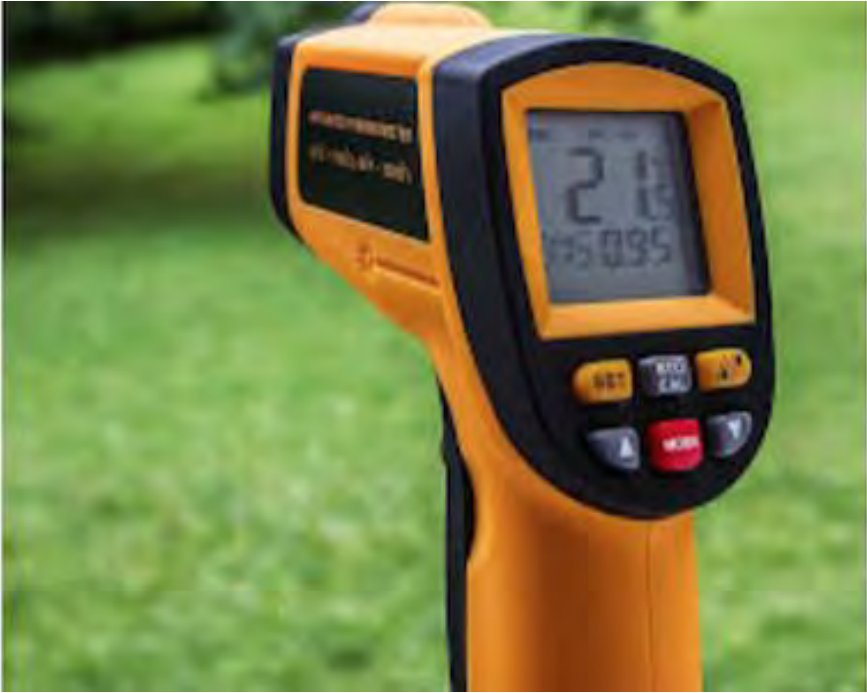
Figure 3. The students used infrared thermometers (IRTs) that are temperature sensing devices using electromagnetic radiation to make non-contact surface temperature readings.
