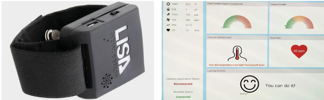
**Figure 2:** The left image shows the LISA wristband, the right image the SmartMonitor app that is connected to the wristband via Bluetooth and that records the physiological data during the training sessions.
