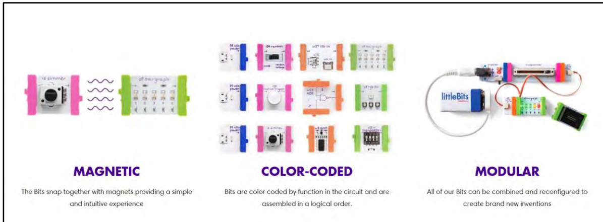
Figure 1. littleBits components and how do they work
