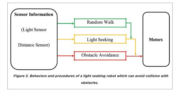
light-seeking) are of no use. That is why, in Fig. 3, we can see that obstacle avoidance behavior is the most basic one (and shown in red color). From the implementation perspective, students might use either or both of IR and ultrasonic distance sensors to detect and avoid obstacles (and other robots).
