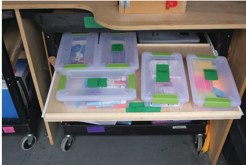
Figure 4. Some shelves slide forward to ease access while in the van. Slides can be locked during transport.
