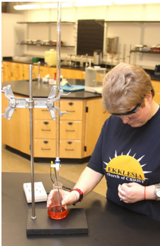
Figure 3. Titration with SALS. The figure exhibits the titration equipment and the SALS probe.
