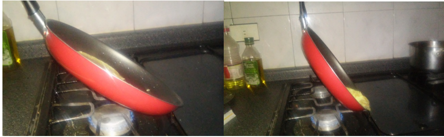
Figure 4. Scrambled Eggs Start to Slide Down When the Angle Is About 45^\circ
