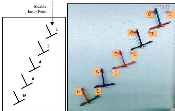
**Figure 2.** Flip-flops are oriented in a line so that inserted marbles will cause a cascading chain reaction. Each gate represents a binary digit, or bit, shown in the diagram on the left. The numbers on the left image show what the bit would represent in base 10, since each gate represents  $2^n$  where  $n$  is the number of marbles. When read from left to right, the number of marbles is represented in binary, seen in the design on the right (USNA STEM Center, 2016a).
