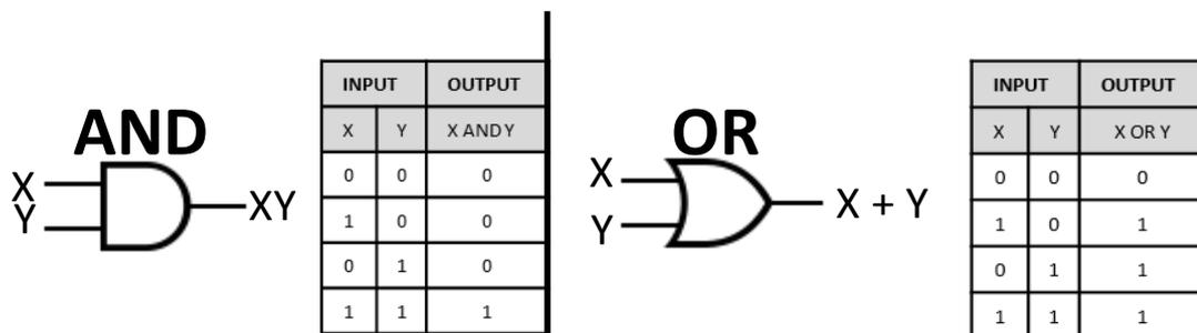
**Figure 3.** Teachers are required to either build an AND or an OR logic gate. Outlined for them are input and output charts of each condition to provide them with background information (USNA STEM Center, 2016b).
