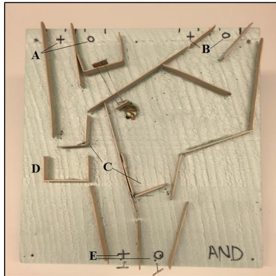
**Figure 4.** Many solutions can come out of the same challenge. An AND gate is represented where there is an x-input (A) and a y-input (B) denoted with either a “0” or a “+” for 1. Flip-flops (C) are used to change the state as marbles travel down the track. Intentional stops (D) are included so that only one ball is returned as an output (E).
