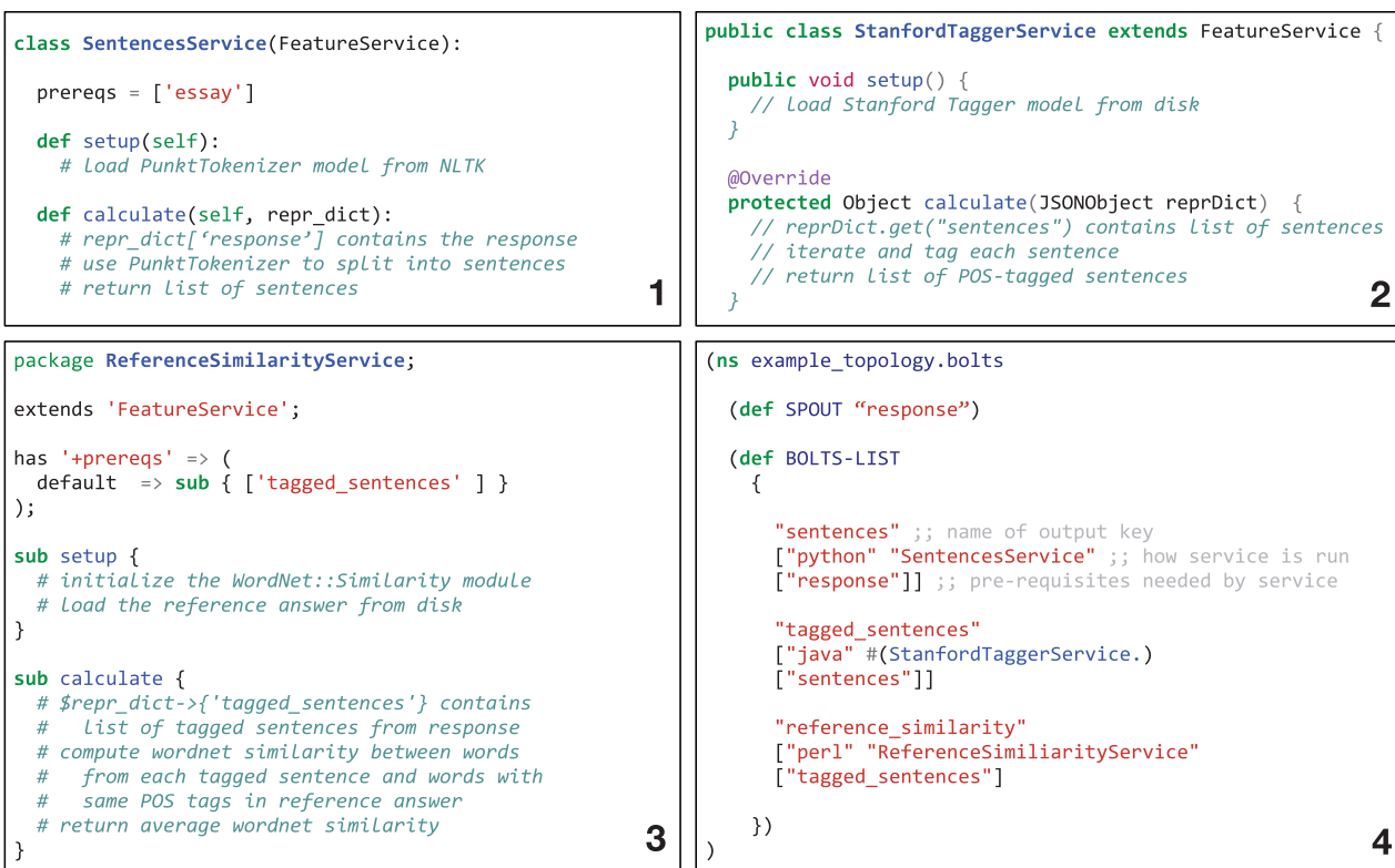
Figure 1 Illustrating Storm microservices and topologies. Boxes 1, 2, and 3 show stubs for three different FeatureService bolts written in Python, Java, and Perl, respectively. Box 4 shows the stub of a topology (written in Clojure) that defines a toy scoring application composed of these bolts.
