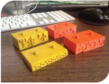
Figure 3. 3-D printed model of sedimentary rock layers
