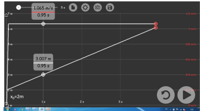
Figure 2. Graphs of the uniform motion of the car as seen by observer A. The velocity-time graph is a horizontal straight line, the position-time graph is a sloping straight line that starts at x_0=2\text{m} .
