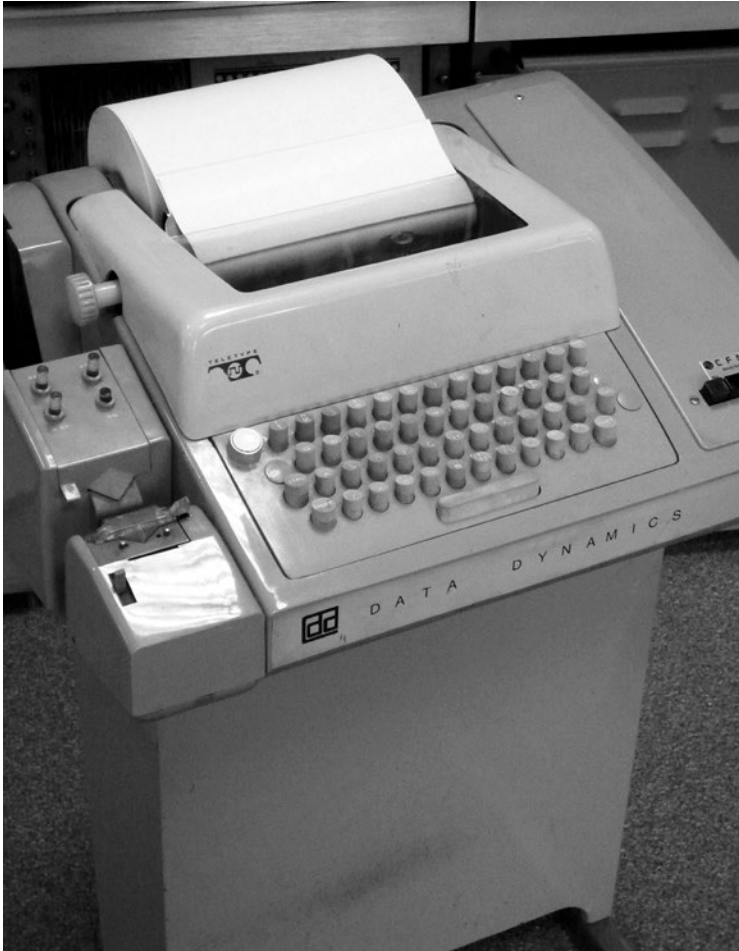
Figure 3. A Teletype Model 33 ASR on display at The National Museum of Computing in 2009. In an email interview, Ken Williams identified this machine as “close” to the machine he used. According to his memory, Williams’s teletype lacked a stand but did have a paper tape reader and an acoustic coupler. Image courtesy of Wikipedia user AlisonW, under Creative Commons BY-SA 3.0
