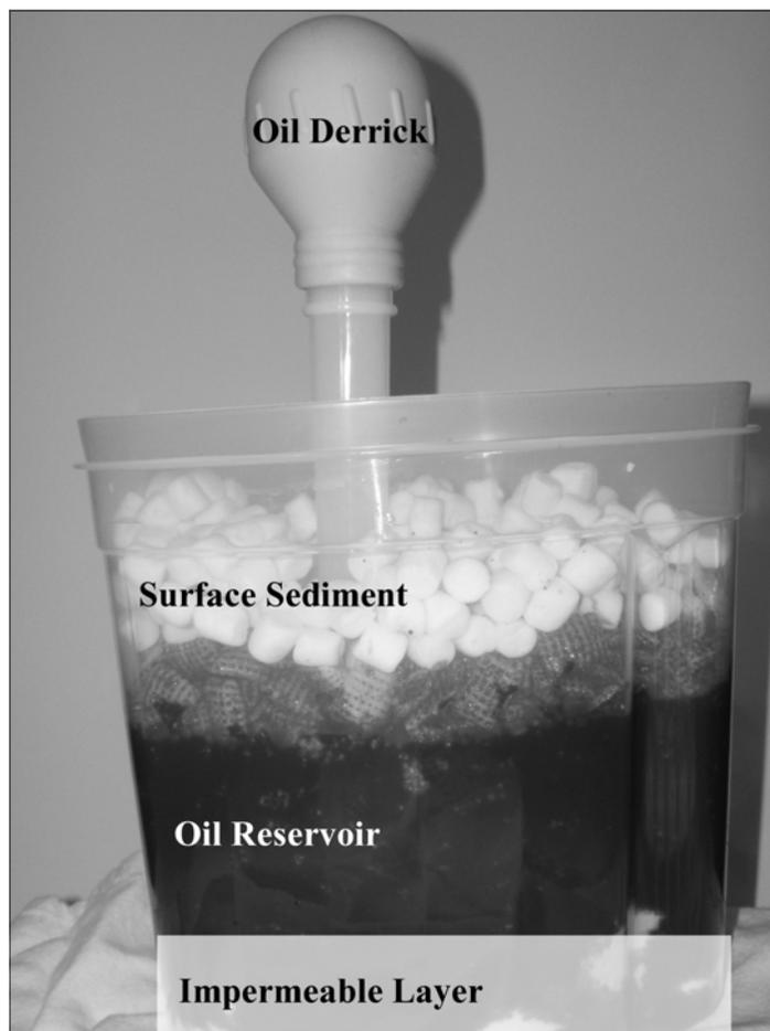
**FIGURE 1. Model of an oil-drilling site on land; the bottom layer is an impermeable smashed cake layer (white added for contrast), the middle layer is the reservoir (porous rice cereal), and the surface layer is made of marshmallows. A baster suctions the chocolate oil from the reservoir.**
