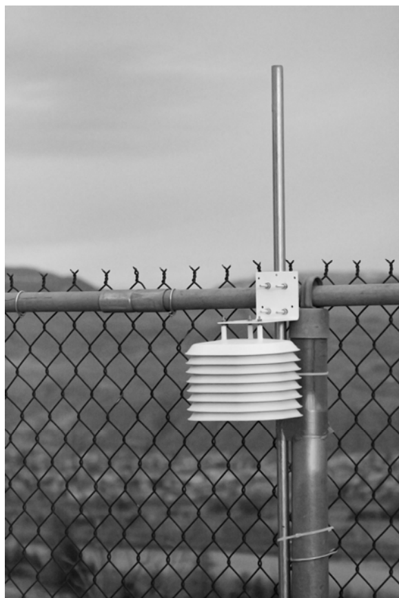
FIGURE 2. A Stevenson screen at Thompson Rivers University, Kamloops, housing temperature and relative humidity probes and a data logger.
