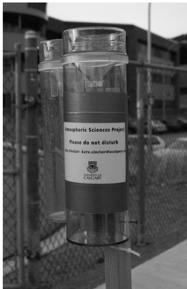
FIGURE 3. A rain gauge installed at Thompson Rivers University, Kamloops.
