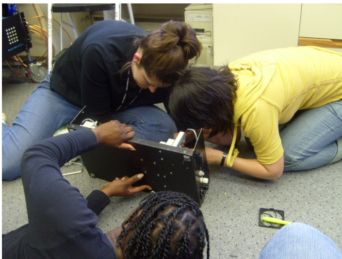
FIGURE 5: Students disassembling an ozone instrument.
