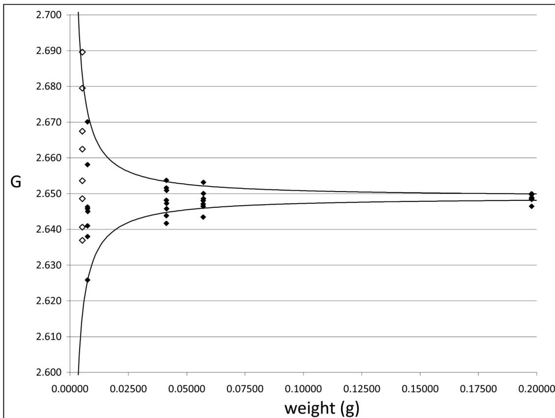
**FIGURE 3. Results of specific gravity measurements for five fragments of a single crystal of pure transparent quartz, with eight separate measurements per fragment. For clarity, open symbols are used for the smallest fragment.**
