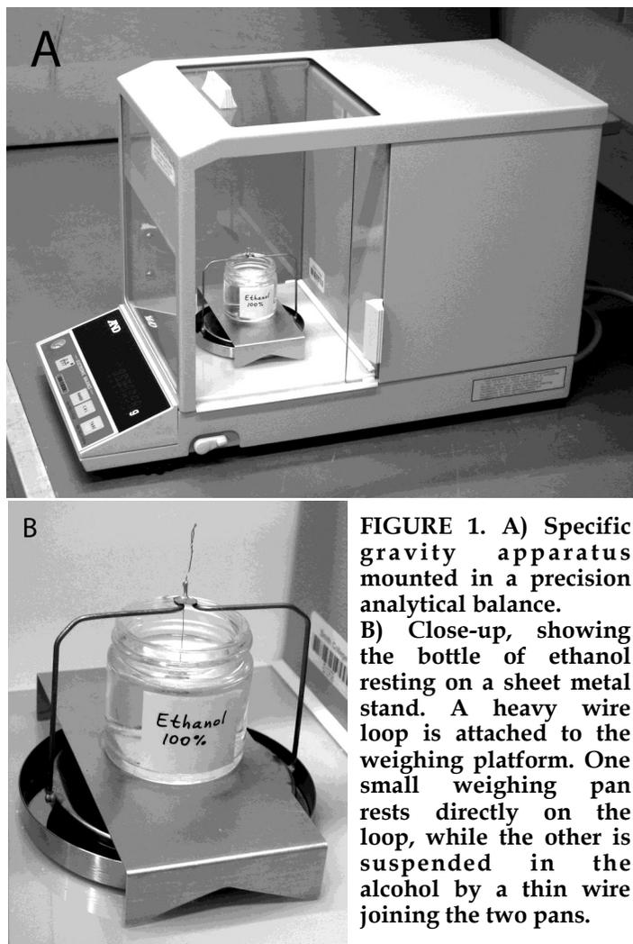
**FIGURE 1.** A) Specific gravity apparatus mounted in a precision analytical balance. B) Close-up, showing the bottle of ethanol resting on a sheet metal stand. A heavy wire loop is attached to the weighing platform. One small weighing pan rests directly on the loop, while the other is suspended in the alcohol by a thin wire joining the two pans.
