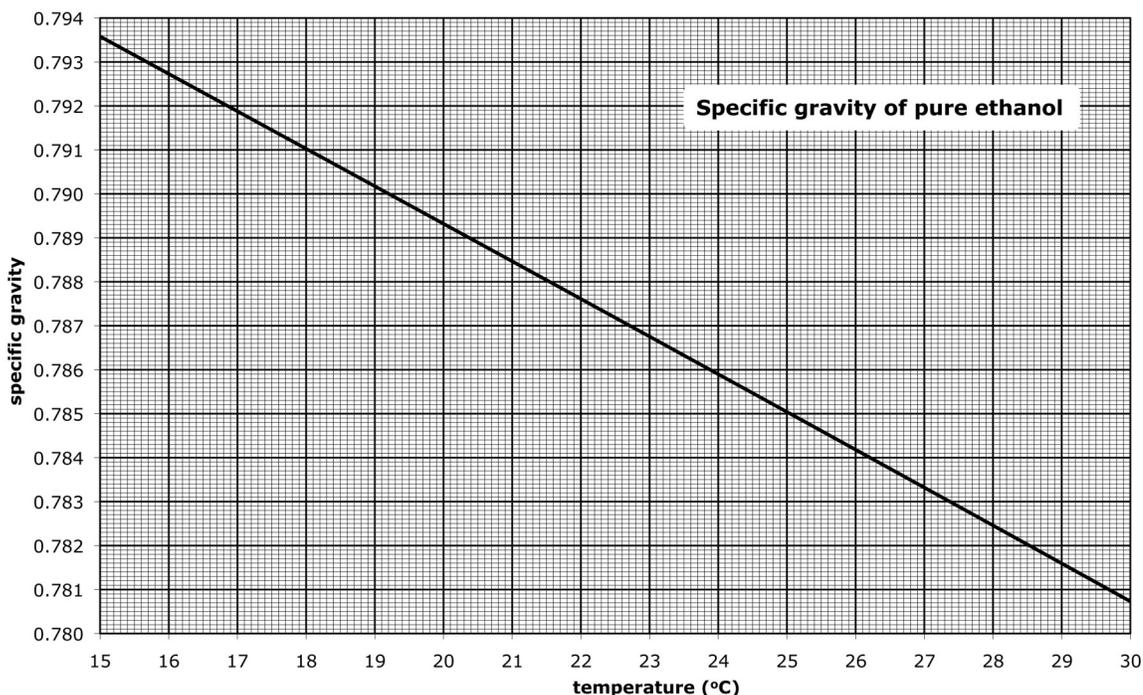
FIGURE 2. Specific gravity of pure ethanol as a function of temperature (data from Lide and Hayes, 2009, CRC Handbook of Chemistry and Physics, 90<sup>th</sup> Edition, page 15-41).
