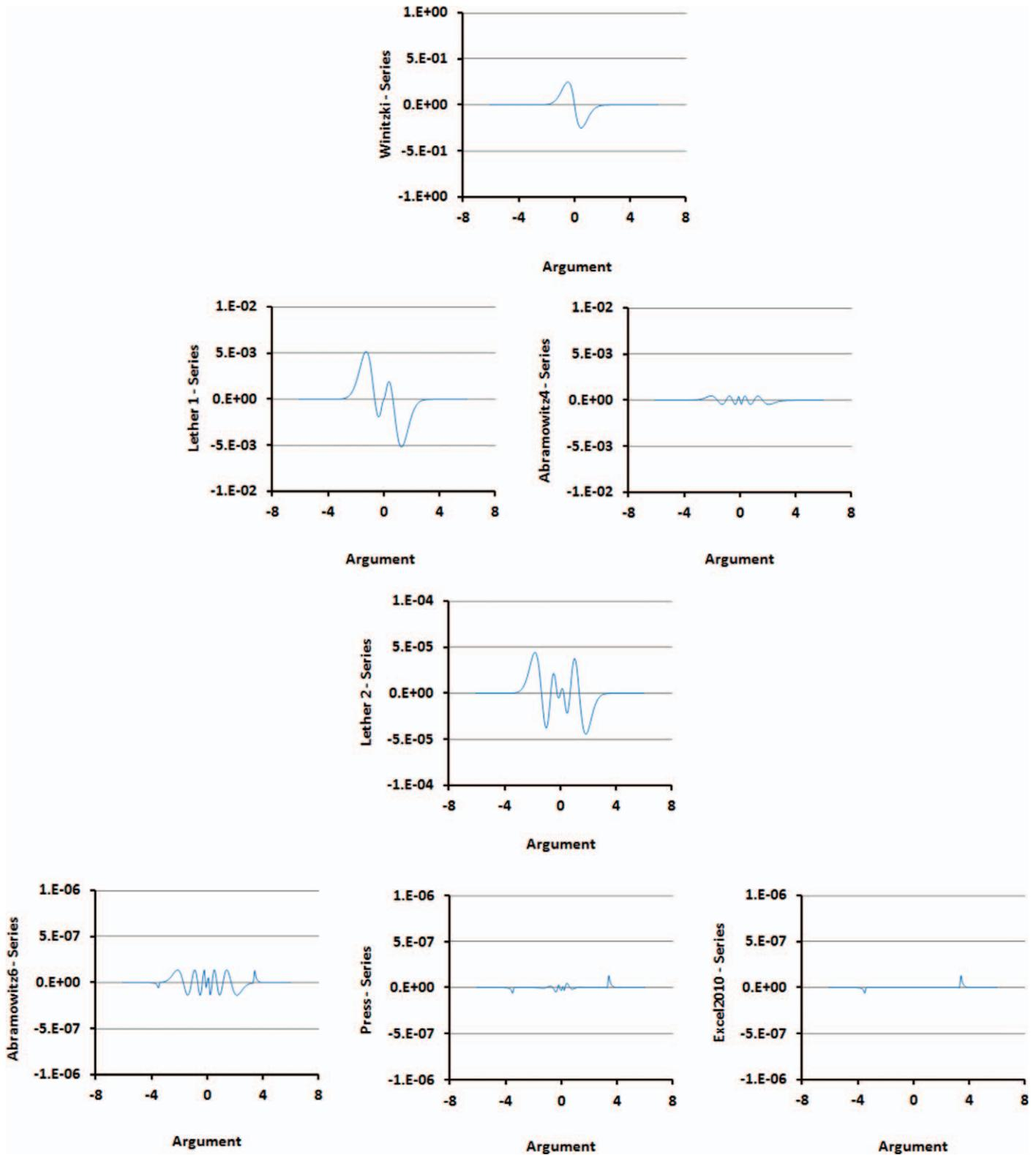
FIGURE 1: Differences between the  $erf(x)$  estimations and the series expansion (first entry in Table I). The  $y$ -axis scales decrease by 2 orders of magnitude with each row of graphs down from the top of the figure. The most accurate estimations are therefore from the algorithms associated with the bottom row.
