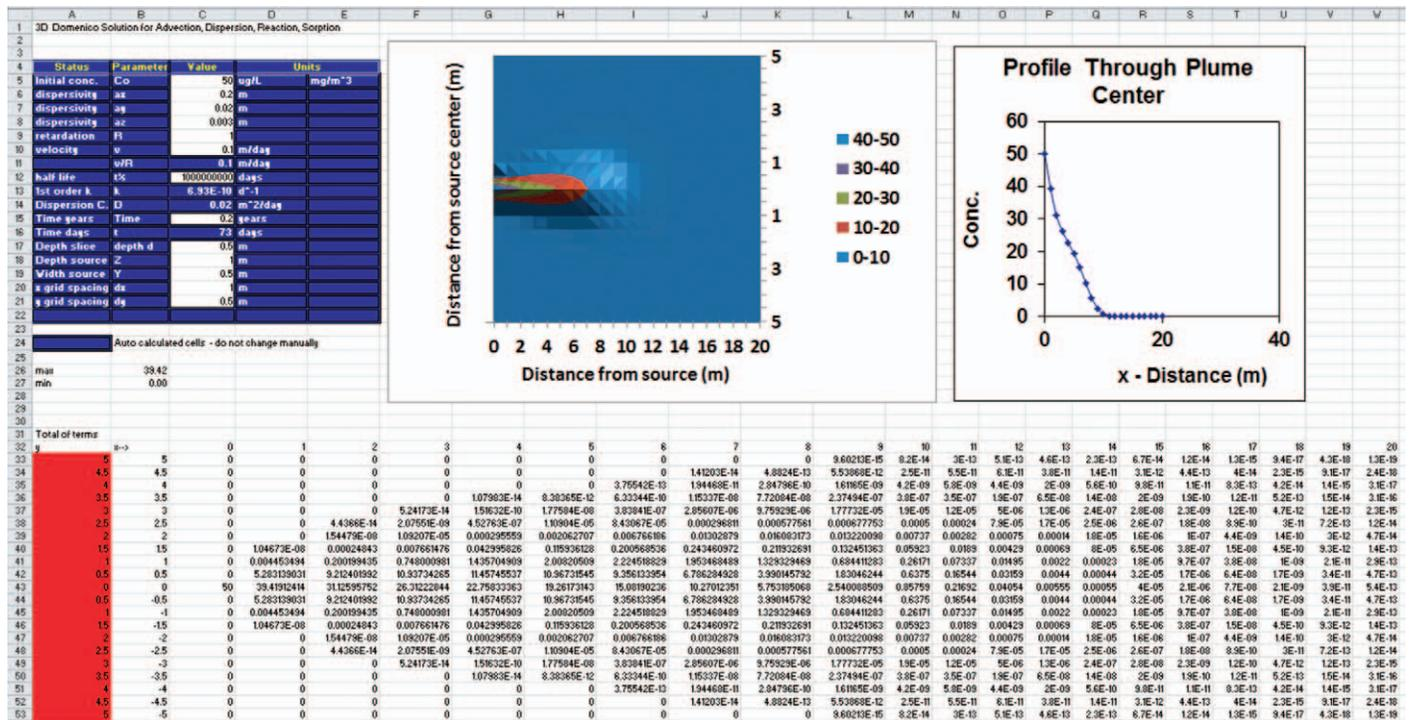
FIGURE 4: Example of input area (upper left), plotted plume slice (upper right), and term area for the equation assembly (bottom, from Eq. 6 in text). Altogether six term areas are present in the worksheet, one corresponding to each term as defined in Eq. 6.
