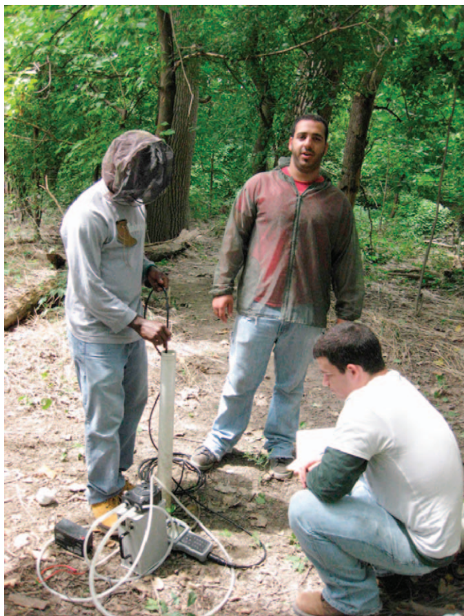
FIGURE 3: Groundwater-monitoring well sampling by students along the lower branch of the Rouge River in Dearborn, MI.
