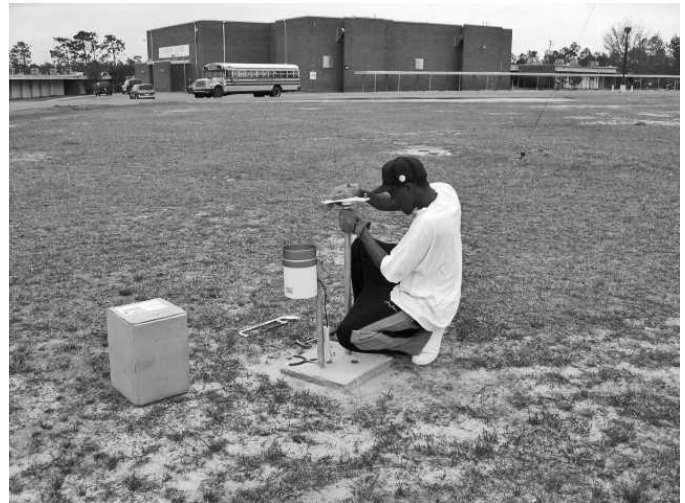
FIGURE 3: Undergraduate meteorology student Quincy Jones helping with installation of rain gauge at a Mississippi Mesonet site.
