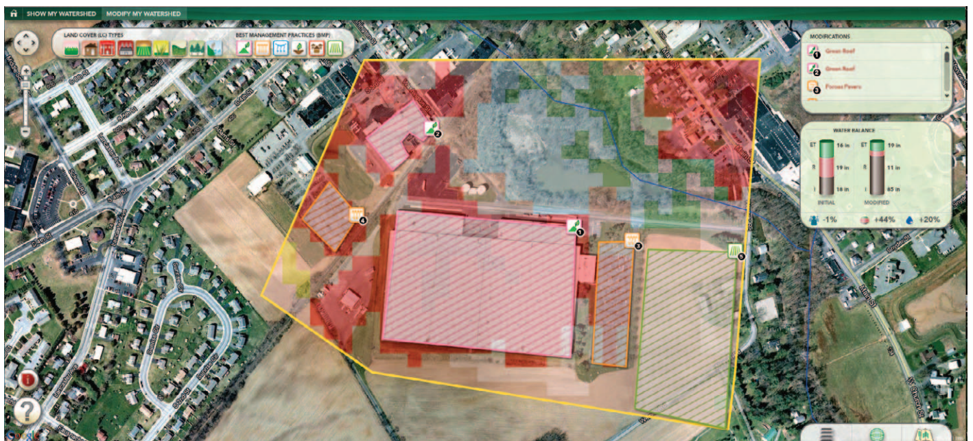
FIGURE 3: Once the student has defined an area and modeled it in the Show My Watershed module, s/he can then modify the area by changing the land-cover type or implementing best-management practices such as green roofs, vegetated infiltration basins, and no-till farming.
