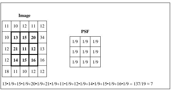
Figure 7. Example of 2D discrete convolution for image
