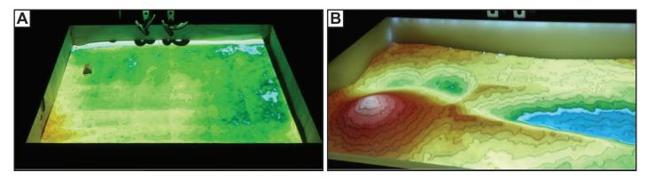
FIGURE 1: View of the augmented reality sandbox. The sand landscape begins as gently sloping surface (A). Subsequently, the sand was sculpted to form a hill, ridge, and a series of depressions (B). The image projected on the sand adjusts in real time to display the new topographic map.
