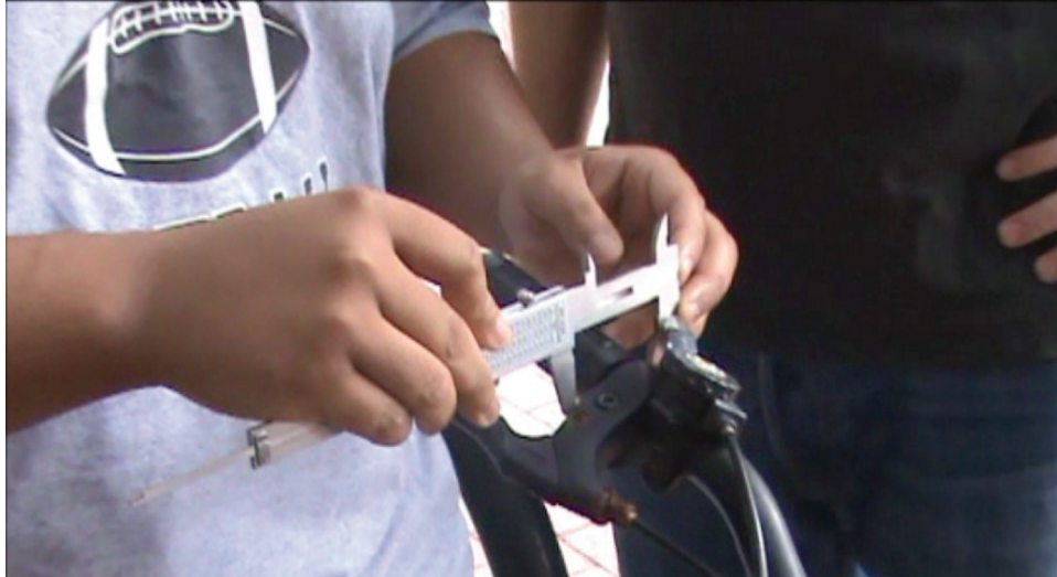
Figure 4. Team Grip-assist Measuring Bike Handles with Calipers
