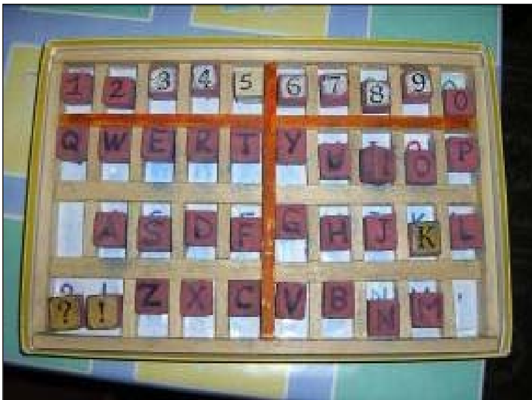
Figure 3. The “keyboard”, with rubber (worn-out) stamps displaying letters of the alphabet and Arabic digits, has a wooden grid that can be taken off to allow for changing and cleaning of the background; this background is printed with letters and numbers and is covered with a transparent slide. Letters and numbers are displayed as for the English computer keyboard (QWERTY), to aid the student in selecting. In math tasks, the letters can be removed and the digits can be removed in spelling tasks.
