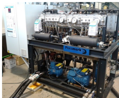
Figure 6. Experimental CO 2 /R134a cascade at the Universitat Jaume I
