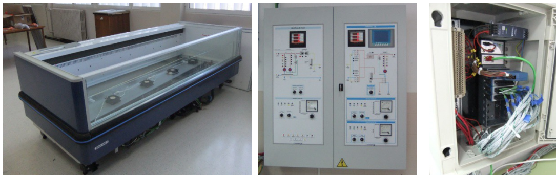
Figure 8. Refrigerated cabinet (left), electrical box (center), DAQ system (right)
