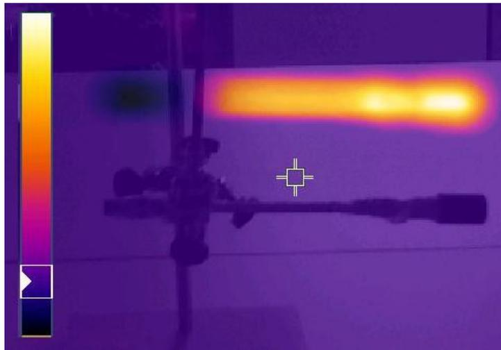
Figure 4. Thermal photography of the vortex tube operating with a cold fraction  $y = 0.75$ .
