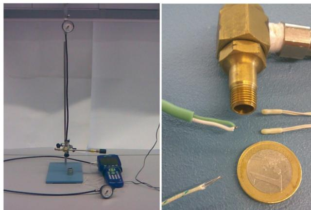
Figure 1. A general view of the laboratory equipment and details of the K-class thermocouples used
