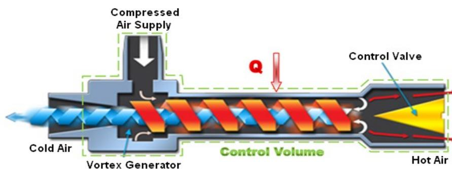
Figure 3. Vortex tube operation and control volume definition
