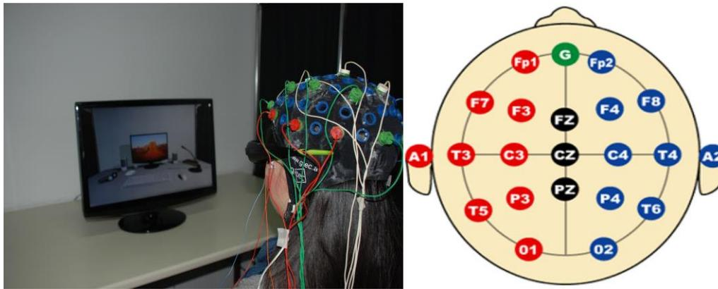
**Figure 2. Left: A student observing the 3D environment. Right: Electrodes' position for EEG recordings (10-20 layout)**
