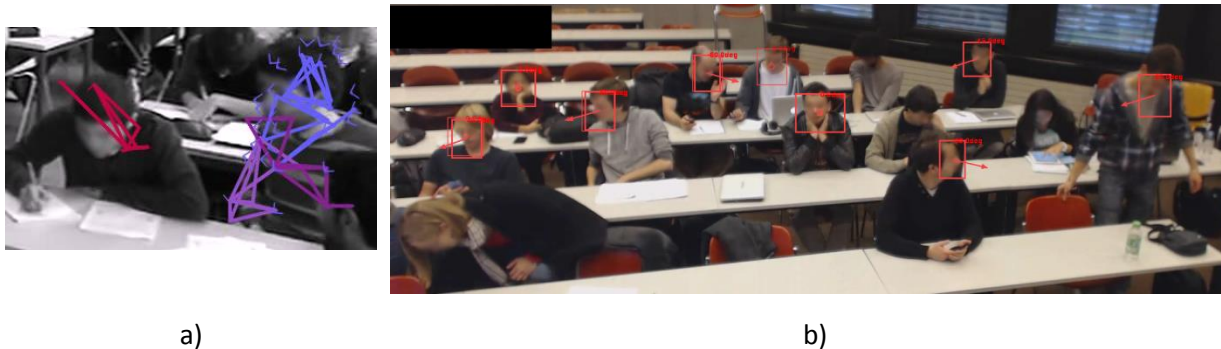
Figure 1: a) Motion vectors visualized on top of the students. Individual vectors are grouped into motion paths depicted as lines of different colours. b) Head detections and estimated gaze directions for a group of students in the classroom.
