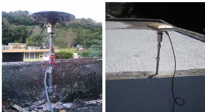
FIGURE 2: Typical “roof-style” GPS monuments installed by students for the first class project, “Where Is My House?”
