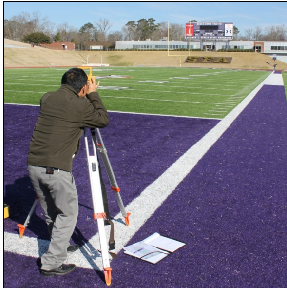
Figure 6. Surveying the dimensions of the football field at Stephen F. Austin State University
