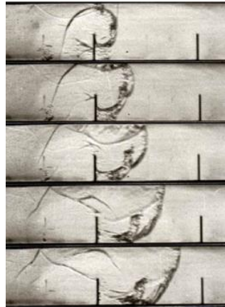
Figure 8. The study of obstacle's influence on detonation wave in channel
