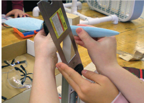
Figure 2. demonstrates students measuring the blade angle with a digital protractor. The information is used in the redesign process to improve turbine output.
