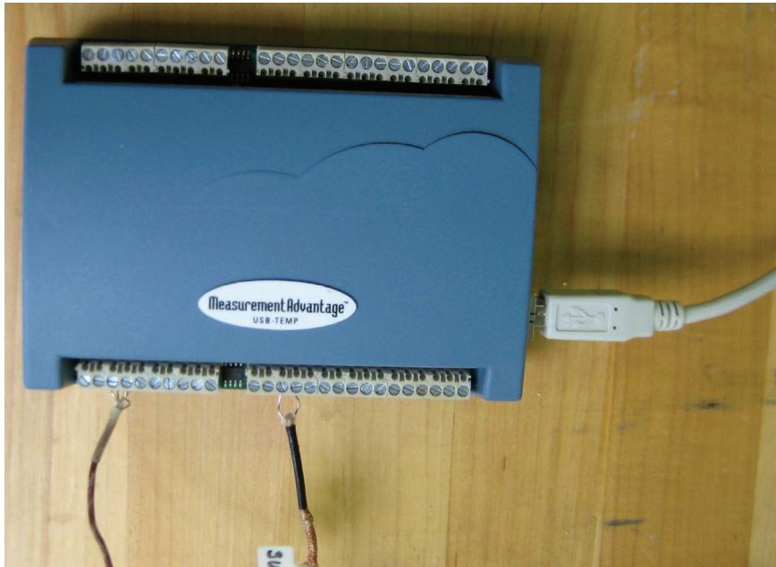
Figure 6. USB-TEMP; a plug-and-play device for temperature measurement. Signal from the two thermocouples is the input to this device; while the output is transmitted through a USB connecting wire to the PC [3].
