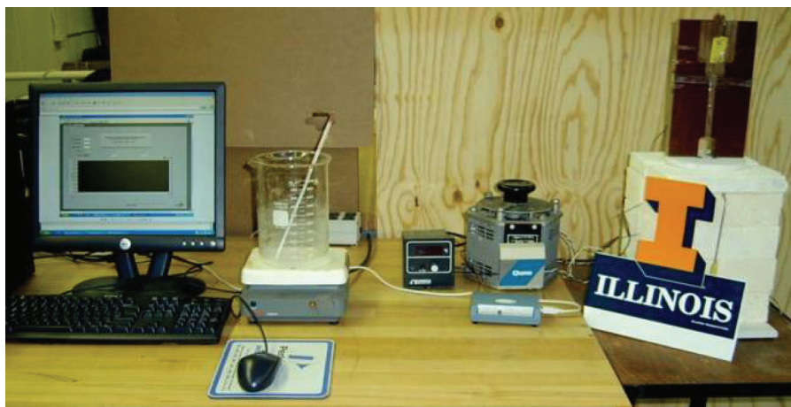
Figure 3. Boiling heat transfer experiment set-up.
