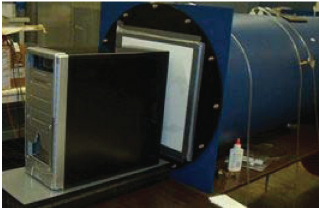
Figure 3. Chassis attached to the Airflow Test Chamber.
