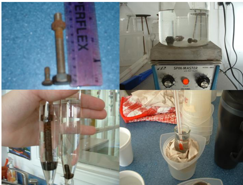
Figure 1. Dr. Spacey's modified procedure for Dr. Boyle. A. (top left) the bolts; B. (top right) the bolts being heated to 100C; C. (bottom left) the bolts in the test-tubes of water; D. (bottom right) one of the test-tubes of water with the bolt added placed in an insulated cup and containing a thermometer for measuring water temperature at specific time intervals (this last step was repeated for both test-tubes).
