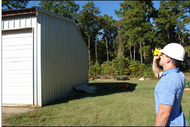
Figure 5. Estimating building feature in the field with a laser rangefinder.
