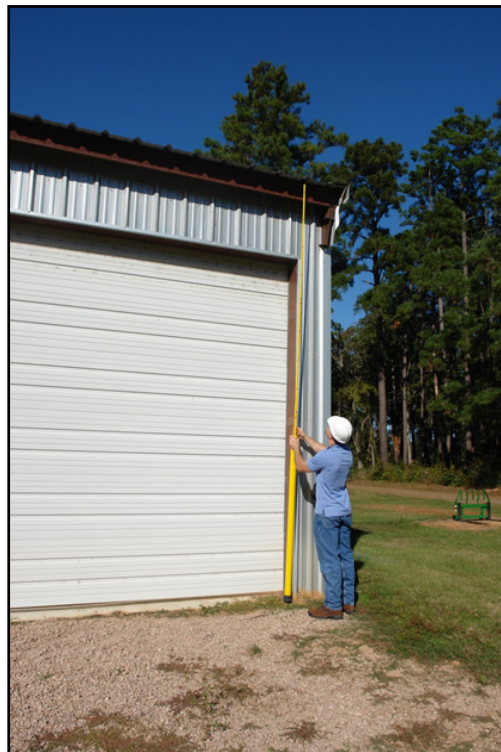
Figure 6. Measuring actual building feature height with a telescopic height pole.
