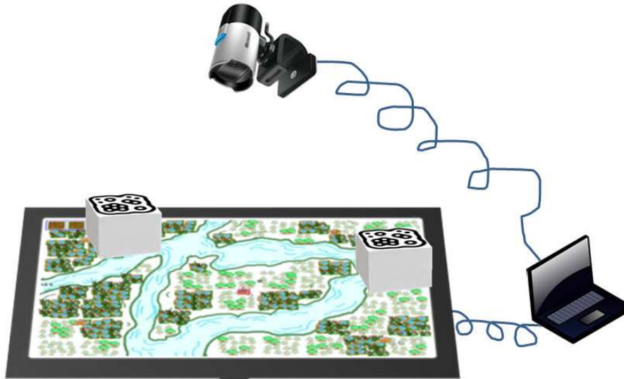
Figure 2: Technical setup for MicroCulture. A webcam (looking down at the game board) captures markers on tangibles; the board is in fact a flat television placed horizontally. A laptop runs the game and outputs on the television screen.
