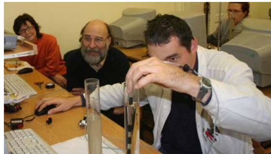
Figure 8. One of the participating teachers, Imre Csiszár, is calibrating the pressure sensor
