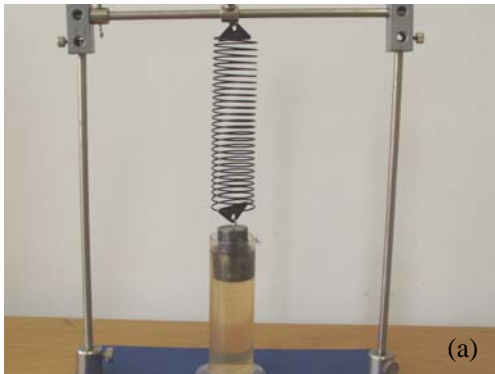
Picture 5. Overdamped oscillation (a) simple model of shock-absorber; (b) strong damping
